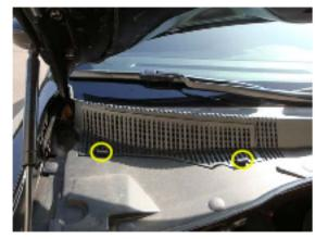
1. The filter is located under the hood. below the windshield on the passenger side. Remove the plastic cover.
