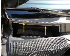
Lift up plastic cover to expose the filter cover. Flip open filter cover to gain access to the filter under it
