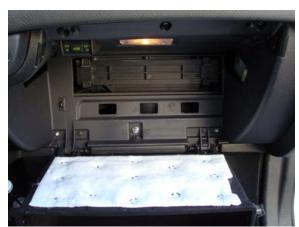
2. Pull down the entire glove box to expose the filter access door behind it.
