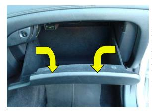
1. The filter is located behind the glove compartment. Push the both sides inwards while pulling down. Allow glove box to swing down on its hinges.
