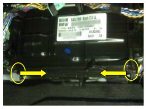
2. Pull down the cover to expose the filters access door. Pull on the locking tab on both side. Set filter access door aside.
