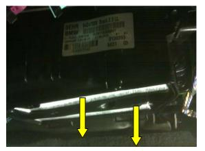
3. Grab the removal flap and slide the both filters out of the housing to remove. Insert new TYC filters, ensuring that the air flow arrow is pointing to the inside of the vehicle.
