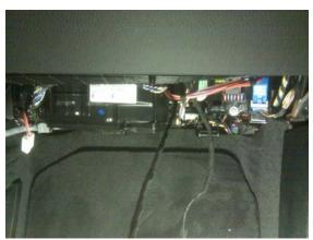
1. The filter is located under the glove compartment. Locate and remove the 4 screws holding up the black foam cover panel.
