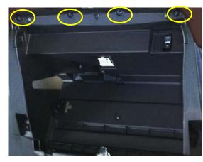
1. The filter is located behind the glove compartment. Remove the four screws along the top of the glove box.
