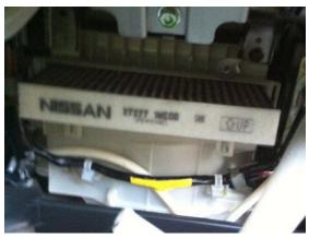
4. Slide out old filter from housing; replace with new TYC filter. Ensure that air flow arrow is pointing up.
