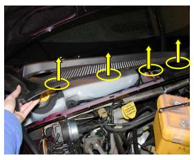
1. The filter is located under the hood, below the windshield at the passenger side. Remove the cowl cover by releasing 4 black plastic captive screws.
