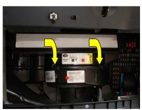
3. Grab the removal flap and slide the filter out from the housing to remove.
