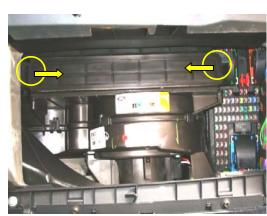
Allow glove box to swing down on its hinges. Filter access door will now be accessible.
