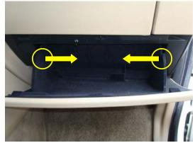
1. The filter is located behind the glove compartment. Push in on the sides of the glove box while pulling down to disengage the latches.
