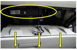
3. Remove the glove box by pulling the entire assembly downwards. Filter access door is now visible.
