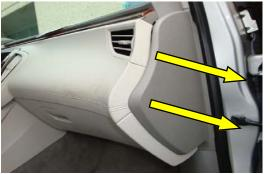
1. The filter is located behind the glove compartment. Remove the end cover located on the side of the dashboard.
