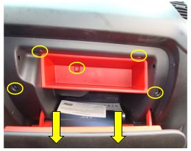
1. The filter is located behind the glove compartment. Remove the 3 screws along the top, 2 in the middle, 3 at the bottom.
