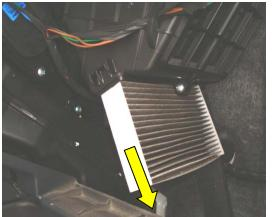
3. Remove the old filter by sliding it down to the right.
