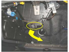
2. Filter access door is now visible. Pull on securing tab and swing filter access door down to open. 10-11 Kia Soul
