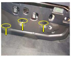
1. The filter is located below the glove compartment. Look below the glove box towards the inside of the vehicle. Locate and remove the 3 plastic screws holding the gray foam cover. Set foam cover aside.
