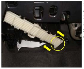
2. The white filter access door is now accessible. Reach in and pull the access door to the left to release. Set filter access door aside.
