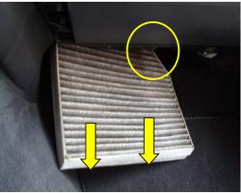
3. Grab the removal flap and slide the filter out of the housing to remove.
