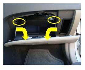
1. The filter is located behind the glove compartment. Push in on the sides of the glove box while pulling down to disengage the latches.
