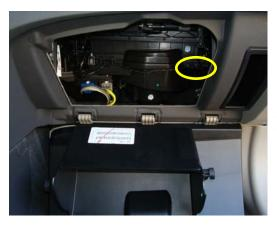
2. Remove the string that is attached to the glove box. Allow glove box to swing down on its hinges. Filter access door will now be accessible.
