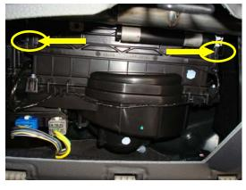
3. Pry away the right and left tabs to remove the filter access door. Then slide the filter out from the housing to remove.
