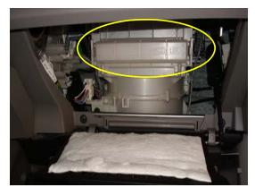
2. With globe box removed, filter access door is now visible.
