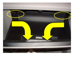
1. The filter is located behind the glove compartment. Push on the sides while pulling down to disengage the latches. Allow glove box to swing down on its hinges. Remove glove box and set it aside.
