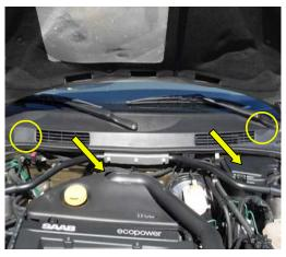
1. The filter is located under the hood, below the windshield. Remove the rubber strip at the edge of the plastic cowl cover, and the 2 screws securing it
