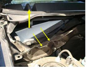
3. Remove old filter from the tray by first lifting it up, then pulling outwards.
