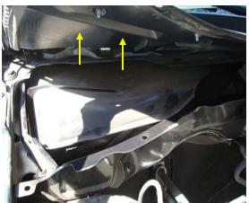
2. Lift up plastic cover to expose the filter cover. Flip open filter cover to gain access to the filter under it
