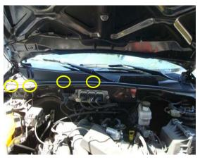
1. The filter is located under the hood, below the windshield on the passenger side. Remove the 4 plastic screws to loosen the cover.
