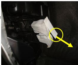
3. Remove filter by grabbing on the white handle and pulling it to
