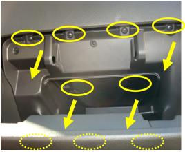
1.The filter is located below the glove compartment. Remove the 4 screws along the top, 2 in the middle, and 3 at the bottom of the glove box. Pull down entire glove compartment and set aside.
