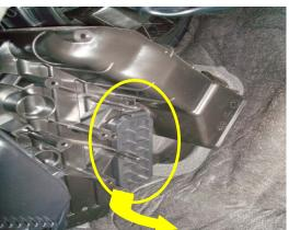
2. Filter access door is located on the left towards the center of the vehicle. Pull on securing tab at the bottom and swing filter access door outwards to remove. Set access door aside.
