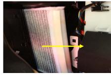
2. Disconnect the 2 electrical connectors behind the glove box to allow it to be completely removed. Set glove box aside.
