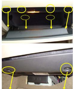
1. The filter is located below the glove compartment. Remove the 4 screws along the top, 2 in the middle, and 2 under the glove box. Gently pull down the loose glove box.
