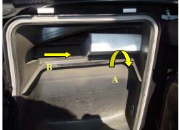
2. Reach in and pull up the first filter on the right, bending the filter slightly. Pull filter towards you to remove (A). Slide the 2nd filter to the right (B), then remove the same way as the first filter.
