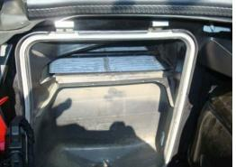
3. Be sure to orientate the new TYC filters where it the Air flow arrow is pointing down. Install the first filter by bending it slightly into the housing and pushing it forward. After inserting first filter, slide it to the left. Install second filter by slightly bending it and pushing it into the housing.
