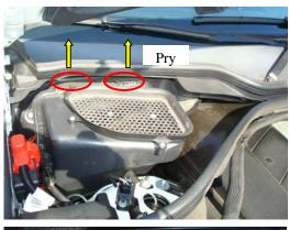
The filter is located under the hood, at the passenger's side. Using a flat head screwdriver, pry open the 2 locking clips on the air box. Lift the loose air box up to remove. Set air box aside.
