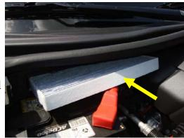
3. Install the new TYC filter by sliding it in. Ensure that the Air Flow indicator is pointing down.
