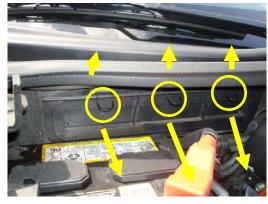
1. The filter is located under the hood, below the windshield on the passenger side. Remove the filter access door by lifting the three clips and pulling it out. Set access door aside.
