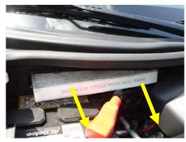
2. Reach into the cavity and slide out the old filter.
