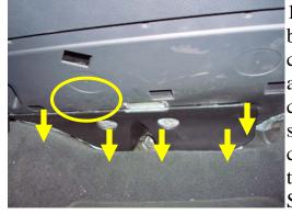
The filter is located behind the glove compartment and can be accessed under the glove compartment. Identify the small piece of black plastic cover, remove it by pulling the entire piece downwards. Set plastic cover aside.
