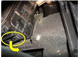
2. The filter access door is located at the upper right corner. Reach in and pull on the locking tab, then pull it to the right to remove. Set filter access door aside.
