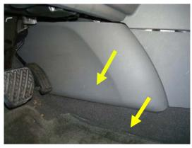
1. The filter is located below the center console and can be accessed by removing the plastic side panel on the driver's side. Pull panel outwards to release. Place panel aside.
