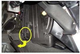
2. Remove the filter access door by pulling the locking tab and swinging it outwards. Place access door aside.
