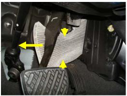
3. Remove filter by squeezing the sides of the old filter softly while pulling it out towards the left.
