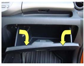
1. The filter is located behind the glove compartment. Push in on the sides of the glove box while pulling down to disengage the latches. Allow glove box to swing down on its hinges.
