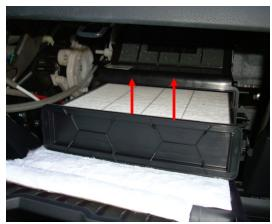
3. Pull up old filter from inside the frame to remove.
