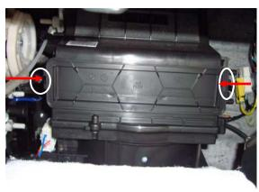
2. Push in on the retaining tabs on each side of the filter frame to release it. Slide the filter frame outwards.
