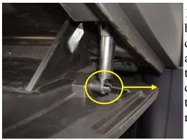
1.The filter is located behind the glove compartment. Pinch the arrow-like head found on the right side of the compartment, then pull the retainer arm to the right to disconnect.
