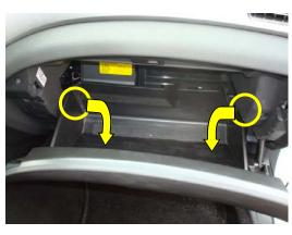
2. Push in on the sides of the glove box latches while pulling down to clear them from the rest of the glove box. Allow the glove box to swing down on its hinges.
