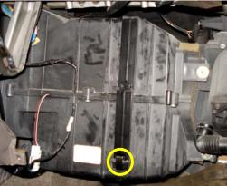
4. Attach the supplied metal clip onto the lower filter and protruding tab of the AC housing.
