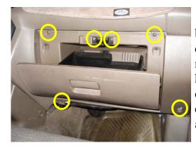
1.The filter is located below the glove compartment. Locate and remove the 6 screws holding the glove compartment. Remove entire assembly and set it aside.
