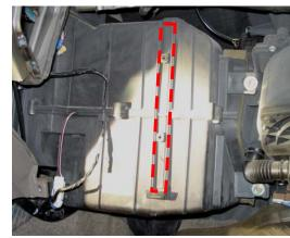
2. If the vehicle is not pre-equipped with a cabin filter a slot will need to be cut out. Cut out the inner panel using the surrounding edge as a guide. Remove and discard cut out material.
