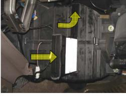
3. Ensure the filter tabs of both filters are facing the bottom.Fully insert the first filter and slide upwards.Follow by sliding the second filter underneath the first.
