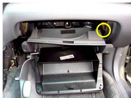
2. While supporting the glove box, disconnect the lamp plug to the right. Fully lower glove box then remove the two knock pins to facilitate reinstallation later. With glove box removed, the filter housing will be visible.
