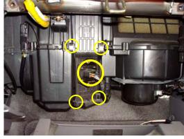
3. Disconnect resistor plug found on filter cover. Release filter cover by removing four clips holding it in place by prying with a flat-head screwdriver. Remove the lower filter first by grabbing its handle. Remove top filter by pulling it down, then out.
