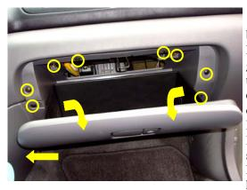
1. The filter is located behind the glove compartment. Push in on both sides of the glove box while pulling down to clear the two knock pins on each side. Allow it to swing down on its rear hinges. Remove the center console's lower right panel by removing screws and pulling it out. Next, remove the screws holding the glove box in place.
