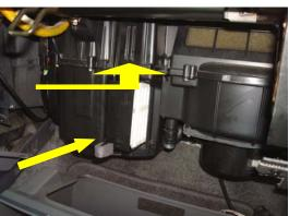
4. Install new TYC filters in reverse order, pushing up the first filter before inserting the second. Make sure the "UP" arrow on both filters are pointing upwards.
