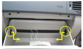
1. The filter is located behind the glove compartment. Push in on the sides of the glove box latches to disengage and remove them.
