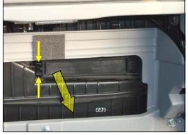
2. Remove damper from glove box by pressing in tabs and pulling away.
