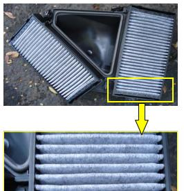
4. Remove filter housing by lifting and pulling away. Turn housing over to reveal the 2 filters. Remove the filter by depressing the 4 retaining clips per filter. Lift the filter up and pull away from the housing. Repeat for the other filter.
