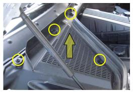
1. The filter is located under the hood. Open the hood, locate the plastic cowl on the passenger side and unlock the 4 retaining bolts by turning them counter clockwise.
