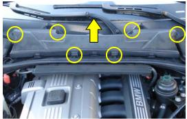
1.The filter is located under the hood, within the engine bay. Open the hood, locate the filter housing panel and remove the 6 bolts.
