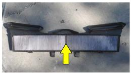
3. Install the new TYC filter by aligning the filter then pushing the filter down into the housing. Ensure the filter housing clips are engaged and locked.
