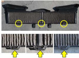
2. Remove filter housing from the vehicle. Turn over filter housing to expose the filter.
