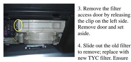
Remove door and set aside. 4. Slide out the old filter to remove; replace with
