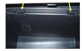
2. Release the filter access panel by depressing the clips and pulling the panel down. Remove panel and set it aside.
