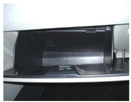
1. The filter is located behind the glove compartment. Open glove box and locate the filter access panel.
