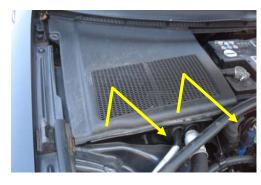
2. Remove plastic cover by lifting upwards then pulling forward. Set plastic cover aside.
