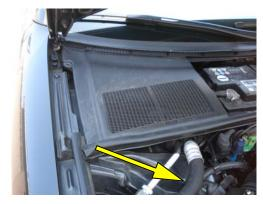
1. The filter is located in the engine compartment, on the passenger side. Begin by removing the weather strip. Pull it away from the plastic covering.
