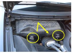
3. Remove the filter cover by releasing the 2 clips at the front, lifting cover and pulling forward. Remove cover and set aside.
