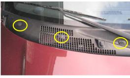
1. The filter is located in the passenger side engine compartment.
