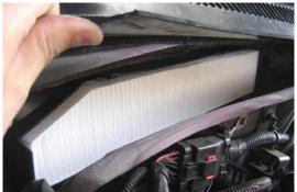
3. Lift the panel in front of the windshield and remove the cover by lifting the 2 tabs at the top and then lift upwards. Remove the cover and place aside.
