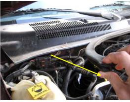
2. Lift hood and pull away weather strip located at the rear of the engine compartment. Remove and place aside.
