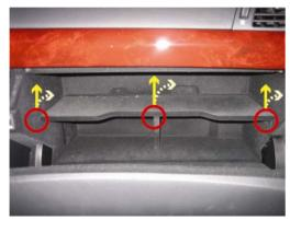
1. The filter is located behind the glove compartment. Open compartment and remove the t-shaped shelf in the glove box by lifting and pulling out the 3 retaining tabs securing the shelf. Remove shelf and set it aside.
