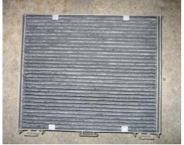
3. Push on the 3 tabs found on the front of the filter frame and lift frame up. Slide frame outwards to remove.
