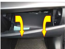
2. Push in on the sides of the glove box while pulling down to clear the latches. Allow the glove box to swing down on its hinges.
