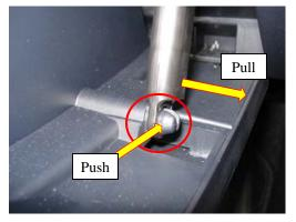
1. The filter is located behind the glove compartment. Open glove box and disconnect the glove box damper by pushing in the retaining clip and pulling damper away.
