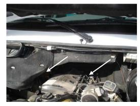
1. The filter is located under the hood, below the middle of the vehicle's windshield. Peel away the foam covering the filter housing.
