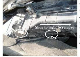
2. Locate and release the 2 clips (one front, one back) securing the filter housing cover. Remove cover by sliding it to the right. Set cover aside.
