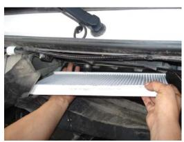
4. Insert new TYC filter into housing. Ensure that the air flow arrow is pointing up.
