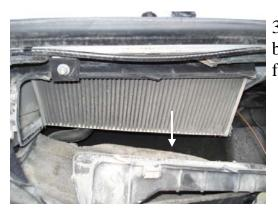
3. The old filter should now be visible. Pull down old filter to remove.
