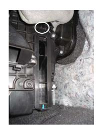
3. Pull on the tab at the top of the filter access door, then push up slightly to release the door.
