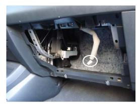
2. Disconnect the electrical connector at the top of the glove box to allow glove box to be completely removed. Set glove box aside.
