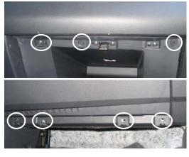
1. The filter is located behind the glove compartment. Remove glove box by uninstalling the 3 screws found at the top, and 4 screws at the bottom.
