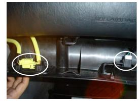
2. Release the 2 wiring connectors behind the glove box cover. Remove glove box cover and set it aside.
