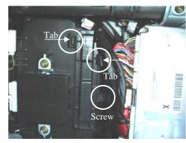
3. Remove the screw holding the filter access door, then push in on the 2 tabs to release. Remove door and set it aside.
