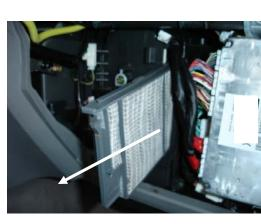
4. Slide out the first filter at the top, then reach in and pull up the second filter in order to slide it out.
