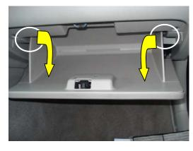
1. The filter is located behind the glove compartment. Push in on the sides of the glove box to clear the retaining latches.
