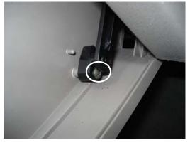
2. Disconnect the damping arm found at the right side by removing the screw. Allow glove box to swing down on its hinges, exposing the filter access door.
