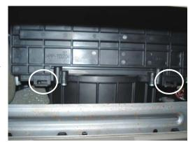
3. Pull up on the two tabs holding the filter access door. Remove door and set aside.
