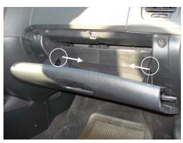
1. The filters are located behind the glove compartment. Remove the latches on each side of the glove box by pushing them inwards. Release the retaining cable and allow glove box to swing down on its hinges.
