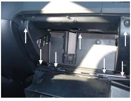
2. Remove the 2 bolts, 4 screws, and 1 nut holding the back panel of the glove box in place. Pull out the entire panel to expose the filter access doors behind it.
