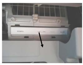
3. Slide out the old filter to remove; replace with new TYC filter. Ensure that the air flow arrow is pointing down.
