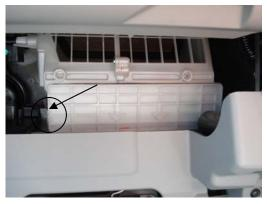
2. Pull on the retaining tab on the filter access door to loosen it. Remove door and set it aside.
