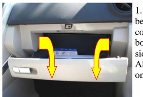
1. The filter is located behind the glove compartment. Open glove box and push in on the sides to clear the latches. Allow box to swing down on its hinges.
