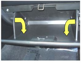
1. The filter is located behind the glove compartment. Open glove box and push in on the sides to clear the latches and allow box to swing down on its hinges.
