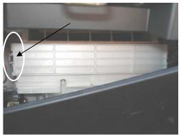
2. Reach in and pull on the retaining tab on the left side of the filter access door. Remove door and set aside.
