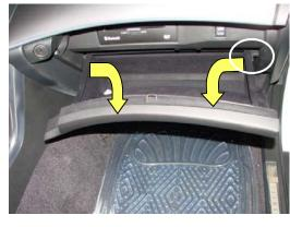
1. The filter is located behind the glove compartment. Open glove box and push in on the sides to clear the latches. Disengage the damping string attached at the right corner. Allow box to swing down on its hinges.
