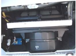
3. Reach in and slide out the old filter. Replace with new TYC filter by sliding it into the housing. Ensure that the air flow arrow is pointing down.
