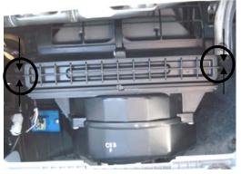
2. Pinch on the 2 securing tabs together on each side to remove the filter access door. Set access door aside.
