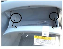
1. The filter is located behind the glove compartment. Slide out the retainer on each side and push them towards the center of the glove box to remove. Allow glove box to swing down on its hinges.
