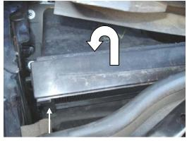
2. Lift up cowl cover to find the filter housing under it. Push on the securing tabs on each side of the housing, and flip up on the cover to gain access to the filter under it.
