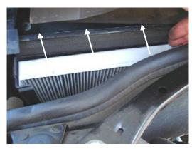
3. Remove the old filter by sliding it up, away from the housing.
