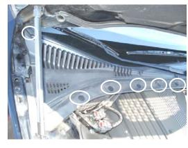
1. The filter is located under the hood, below the cowl cover at the passenger side. Locate and remove the plastic pins securing the cowl cover.
