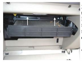
3. Remove old filter from the frame by lifting it up. Insert new TYC filter into frame, ensuring that the air flow arrow is pointing down.
