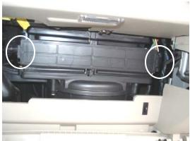
2. Pull on the 2 tabs on the sides of the filter access door, slide out the filter frame. The filter is installed inside the frame.
