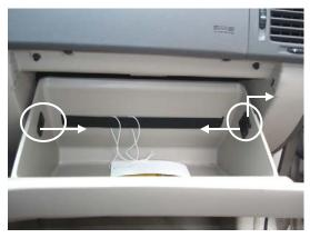
1. The filter is located behind the glove compartment. Push in on the sides of the glove box latches to disengage and remove them.
