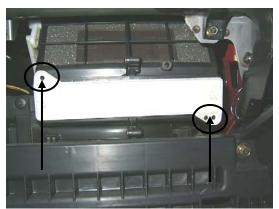
3. Insert in new TYC filter, ensuring that the Air Flow arrow is pointing down, and that the frame is aligned with the housing's mounting screw (at opposite corners). Screw in the mounting screws to secure filter.
