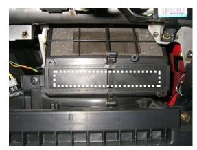
2. For first-time installation\*, the filter housing is sealed. Use a sharp knife to cut the cover along the lines to form a rectangular opening. Remove and dispose the cut out cover.
