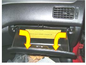
1. The filter is located behind the glove compartment. Push in on the sides of the glove box while pulling down to disengage the latches. Allow box to swing down on its hinges.
