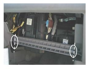
2. Cut the plastic cover along the dotted lines shown and remove it. Dispose off plastic cover, it is no longer needed. This exposes the metal cross bar under it. Locate and remove 2 additional bolts securing bar. Remove and set it aside.
