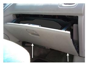
1. The filter is located behind the glove compartment. Unscrew the 2 screws at the bottom of the glove box cover to loosen the it. Remove glove box and set it aside.
