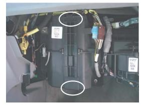
3. The filter access door is now accessible. Pull on the top and bottom tabs to release door. Remove door and set it aside.
