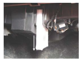
4. Replace with new TYC filters in the same location. Ensure that the Air Flow arrow is pointing towards the driver's side for both filters.
