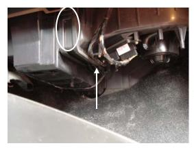
2. Locate the single bolt securing the filter access door and remove it. Pull on the tab at the top of the access door to release it. Remove door and set it aside.
