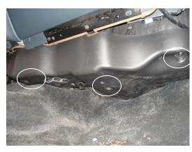
1. The filters are located under the glove compartment. Locate and remove the 3 screws securing the plastic cover. Remove cover and set it aside.
