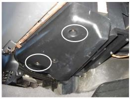
1.The filter is located below the glove compartment. Locate and remove the 2 screws holding up the plastic cover in front of the filter access door. Remove cover and set it aside.
