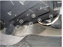
2. Locate and remove the 6 screws securing the filter access door. Remove door and set aside.
