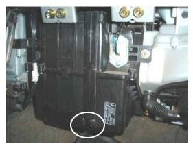
3. Remove the clip that holds the filters in place. Slide out both of the old filters. Replace with new TYC filters, ensuring that the Air Flow arrow is pointing to the driver's side for both filters.
