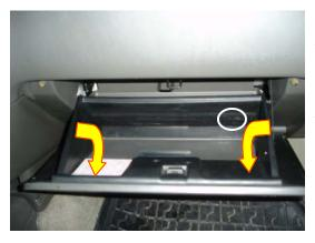
1. The filters are located behind the glove compartment. Push in on the sides of the glove box while pulling down to disengage the latches. Remove the retaining string that is attached to the glove box.
