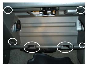
2. Allow glove box to swing down on its hinges. Remove the hinges and disconnect the glove box. Set it aside. Locate and remove the 4 screws holding up the glove compartment cover and remove cover.
