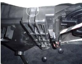
2. Pull down the plastic cover to expose the filter access door. Pull on the retaining tab to remove door and set door aside.
