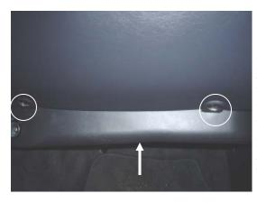
1. The filter is located under the glove box. Remove the 2 screws holding up the plastic cover panel and pull on the tab found at the middle of the cover panel.
