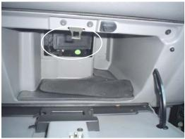
1. The filters are located behind the glove compartment. Open the glove box, remove the plastic cover to expose the filter access door.
