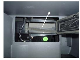
2. Pull on the filter access door and it will swing open. Pull out the first filter by sliding it out towards you.
