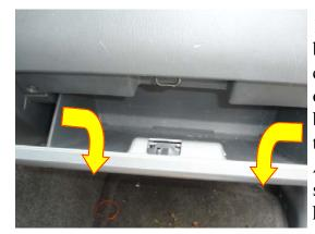
1. The filters are located behind the glove compartment. Push in on the sides of the glove box while pulling down to disengage the latches. Allow glove box to swing down on its hinges.
