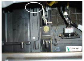
2. Pull on the tab at the top of the filter access door to release. Pull up the door to release it from its bottom groove. Set door aside.
