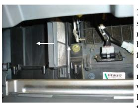
3. Grab the handle and slide out the first filter to remove. Lift up the bottom filter to where the first filter was, and slide it out the same way. Insert new TYC filters the same way, ensuring that the Air Flow arrow is pointing towards the driver's side.
